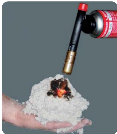
Test hořlavosti Climatizeru Plus
